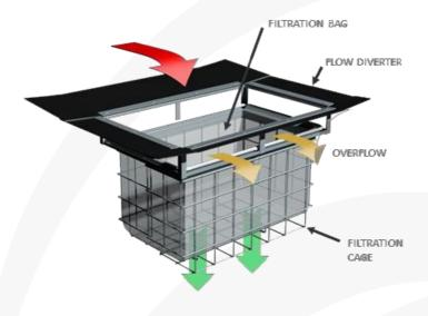
During larger rain events the large flows overflow slots in the flow diverter of the OceanGuard ensure that the conveyance of stormwater is not impeded thus eliminating the potential for surface flooding. As the flow subsides, the captured pollutants are held in the OceanGuard Filtration bag dry. The waste then starts to dry which reduces the magnitude of organic material decomposition transitioning between maintenance intervals.
