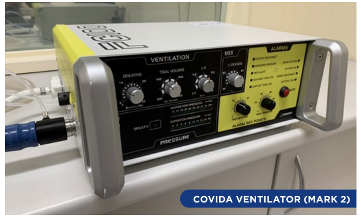
CLINICAL SIMULATION TESTING OF EARLY PROTOTYPE COVIDA VENTILATOR
