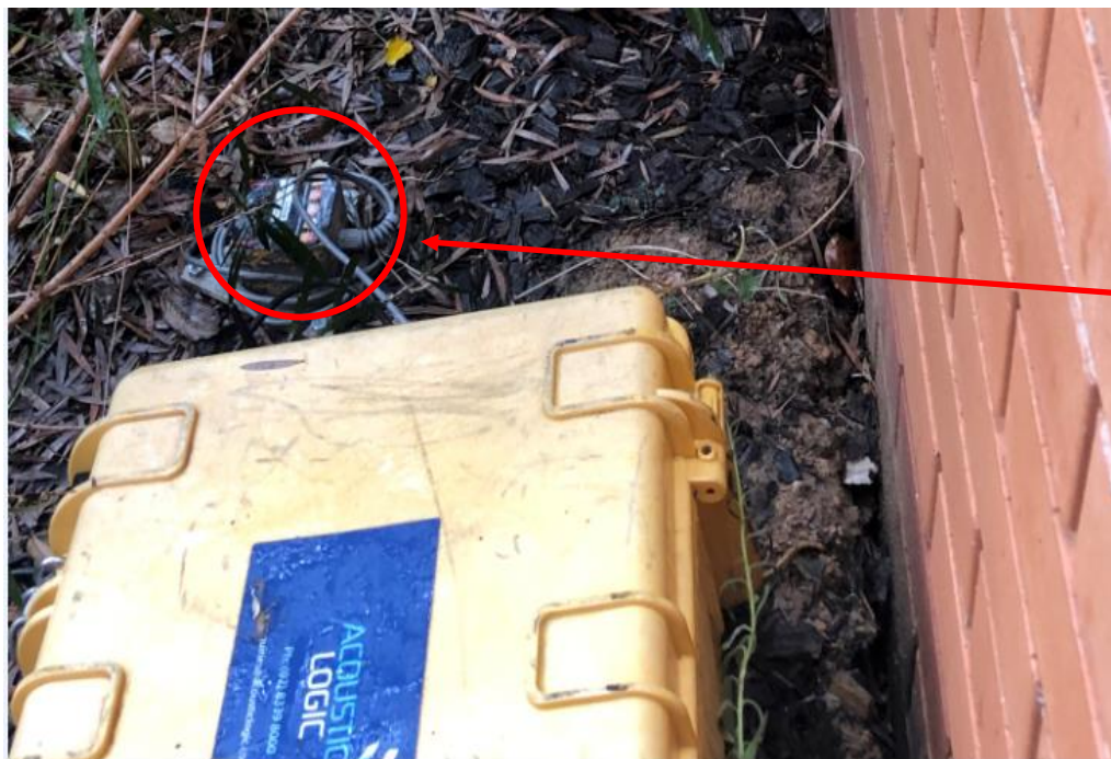
Figure 3: Vibration Monitor installed within Brain Injury Unit Garden Bed
