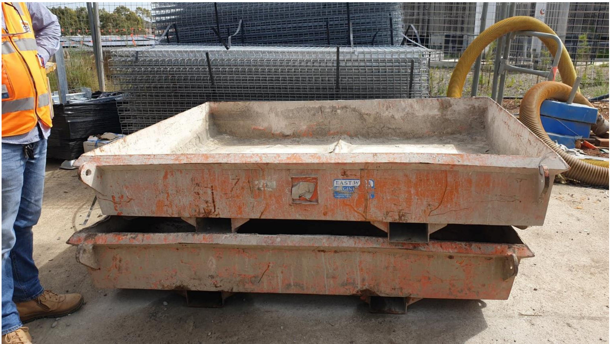
Photo 13: CoC C33 – Concrete washout trays
