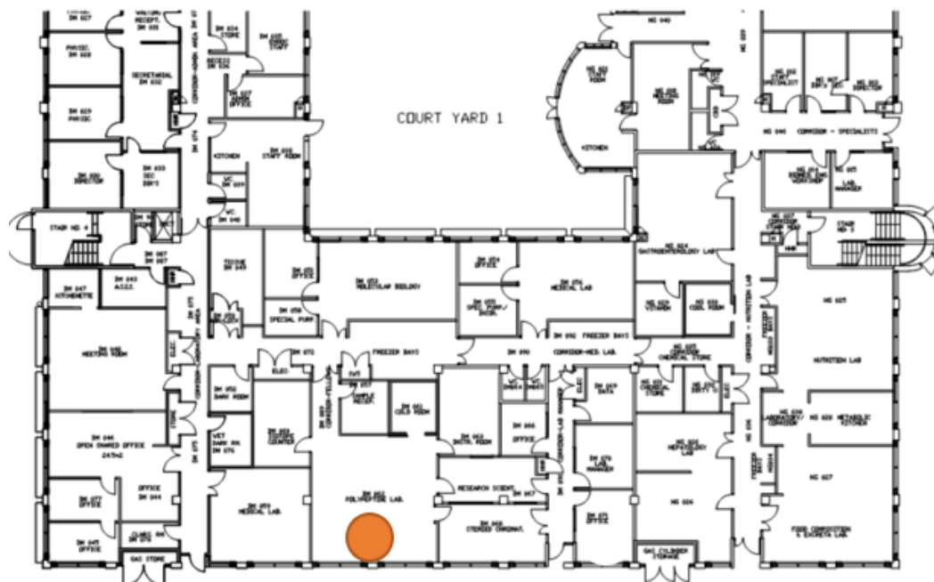
Figure 2: CHW - L1 Lab vibration monitor location shown in orange
