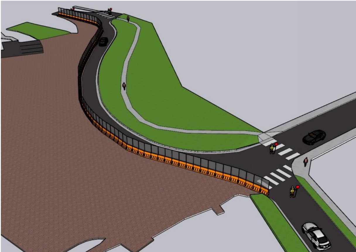
Figure 8: Stage 3 – Southbound Construction Part 2
