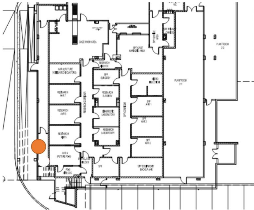
Figure 3: KR - Animal House vibration monitor location shown in orange
