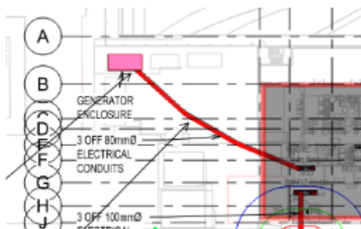
Figure 4-11: Proposed Generator location in the Loading Dock Area and the inground conduit reticulation
