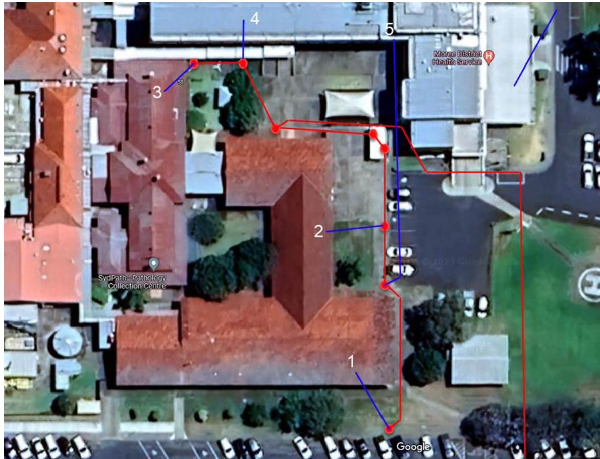
Figure 4-8: Location of the Existing fibre and copper pathway as per DBYD (red denotes conduits and blue denotes cable entry to building, 2 is the approximate location of the existing CD)
