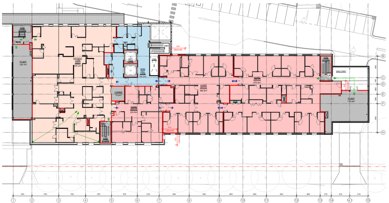
Fire Compartment First Floor Plan
