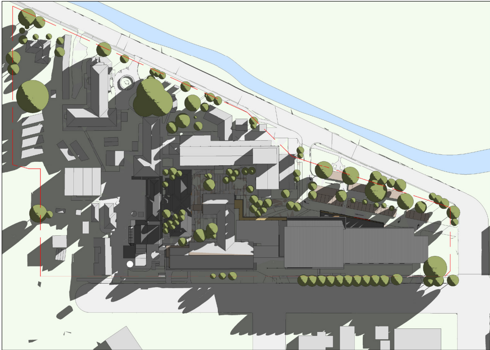
1 Proposed Site Plan Shadow Analysis-Winter 9am SCALE: 1:1000
