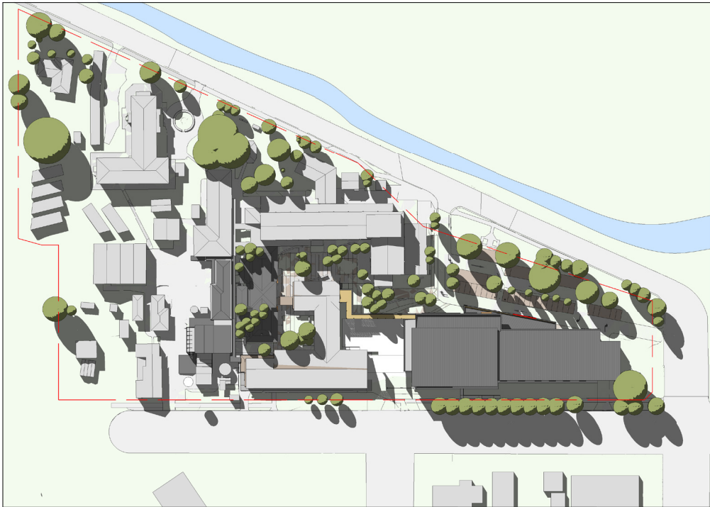
3 Proposed Site Plan Shadow Analysis-Winter 3pm SCALE: 1:1000
