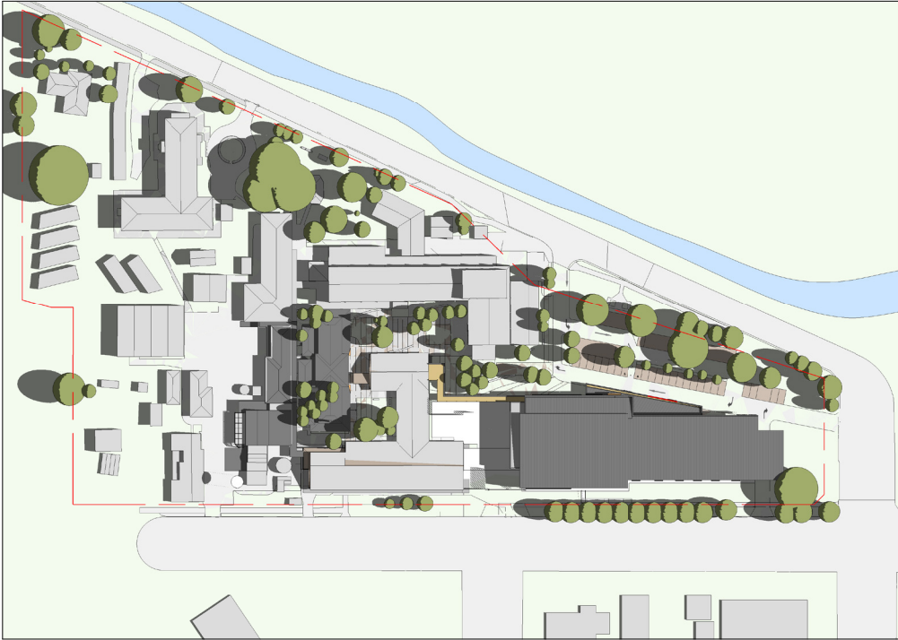
1 Proposed Site Plan Shadow Analysis-Summer 9am SCALE: 1:1000
