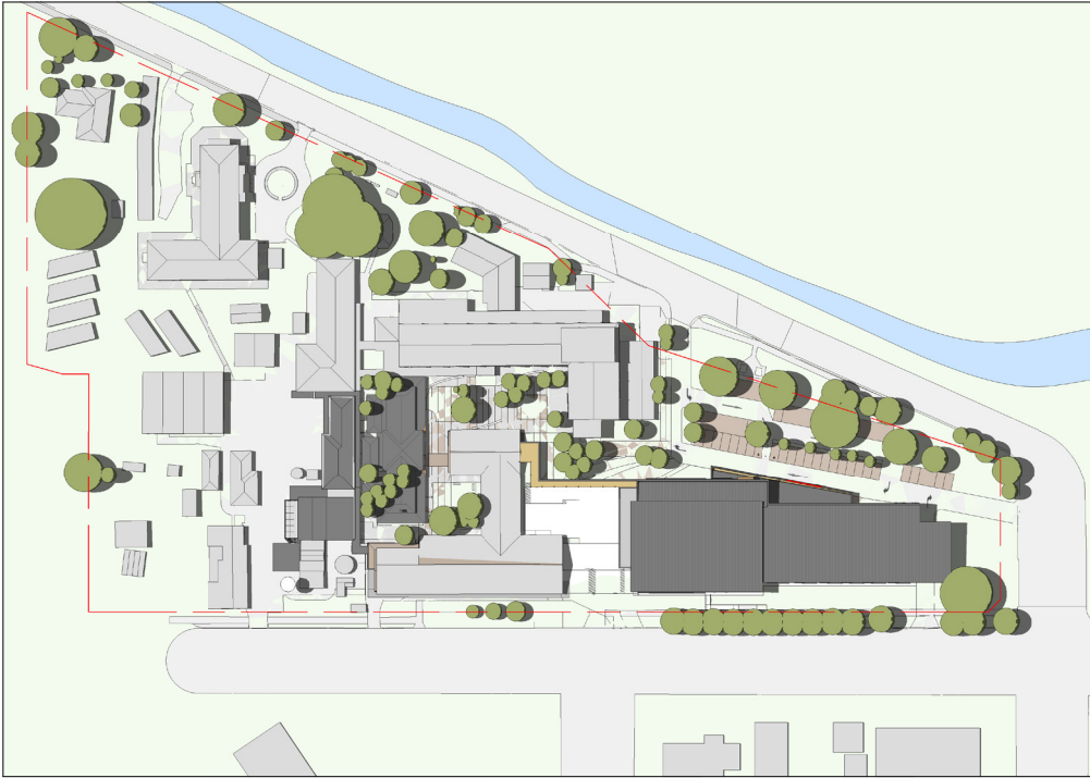
3 Proposed Site Plan Shadow Analysis-Summer 3pm SCALE: 1:1000
