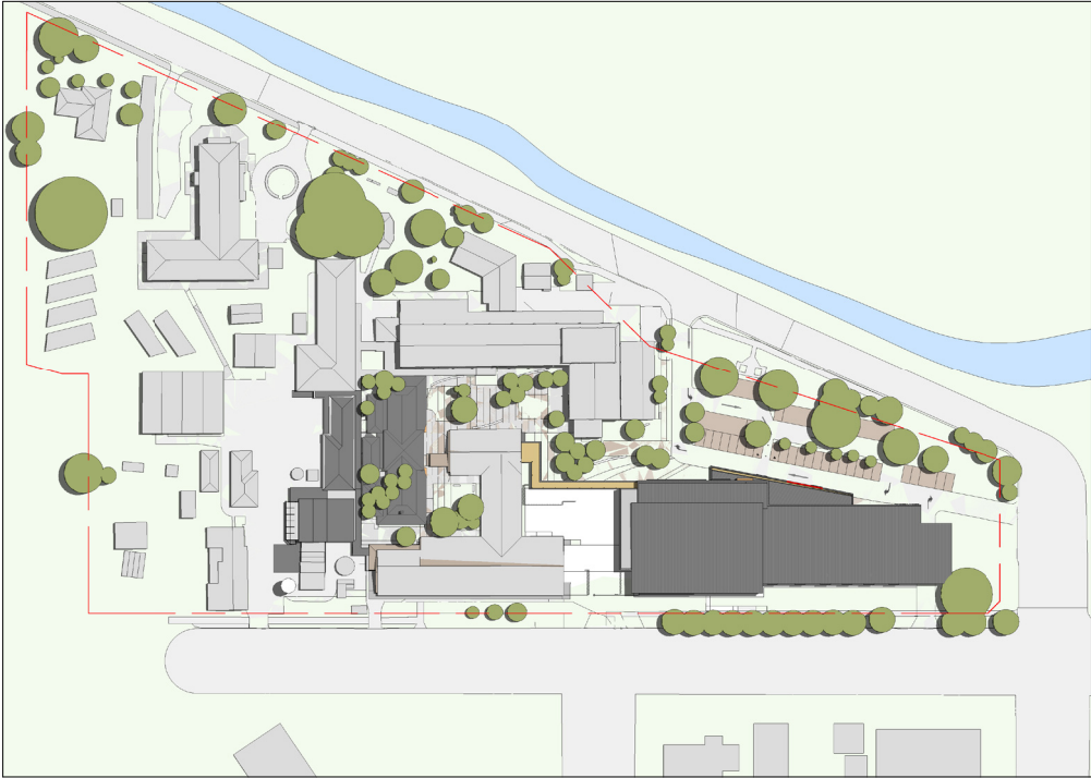
2 Proposed Site Plan Shadow Analysis-Summer 12pm SCALE: 1:1000
