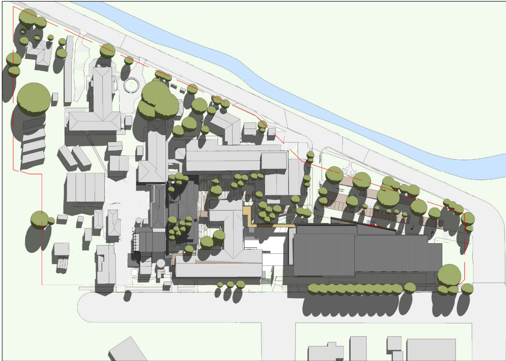
2 Proposed Site Plan Shadow Analysis-Winter 12pm SCALE: 1:1000
