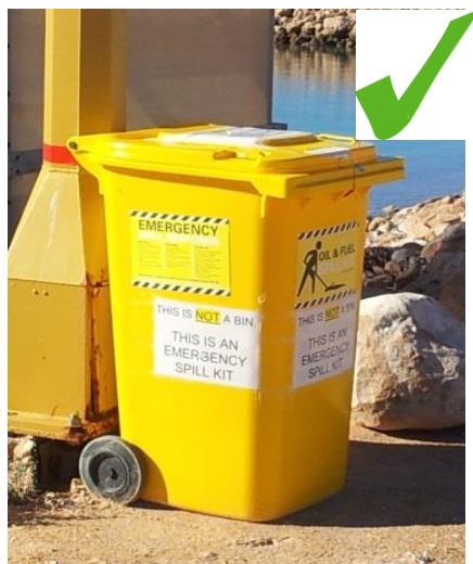
Spill kit easily accessible and clearly marked
