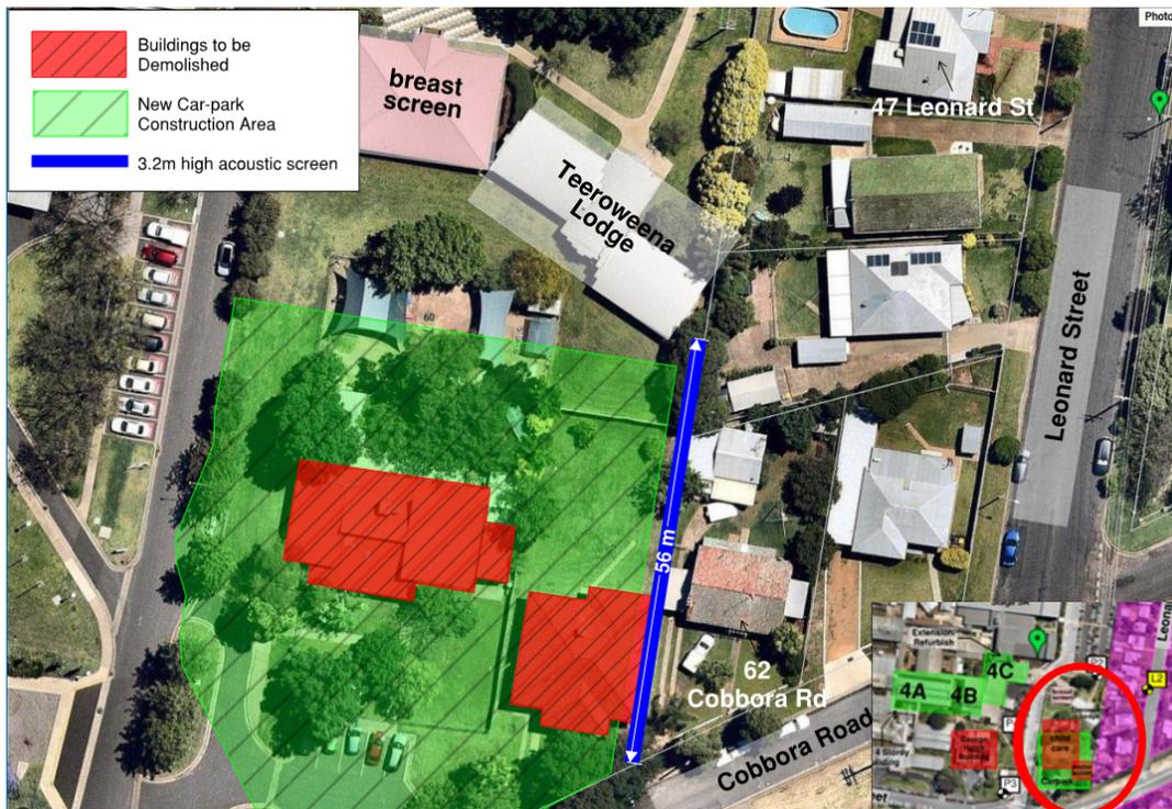
To assess noise and vibration impacts during construction, a number of typical scenarios using various type of equipment have been used. Assumptions of typical equipment associated with the works for phases 1 – 6 have been made in Section 4.2. The equipment noise levels are extracted from AS2436:2010 “Guide to Noise and Vibration Control on Construction, Demolition and Maintenance Sites” and Department of Environmental and Climate Change NSW – Interim Construction Noise Guideline (July 2009).
