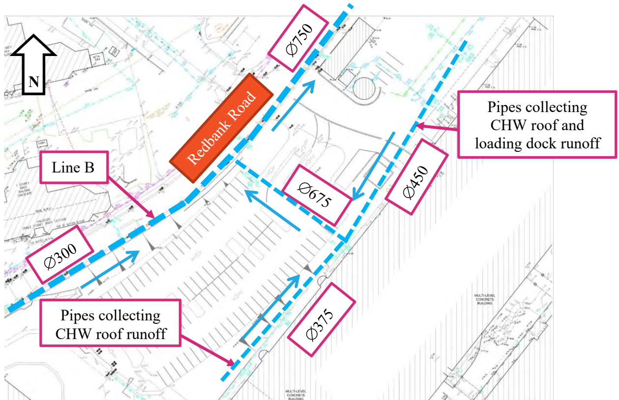
Figure 4 - Extract of CHW Site Survey – Line B (LTS Lockley, 2020)
