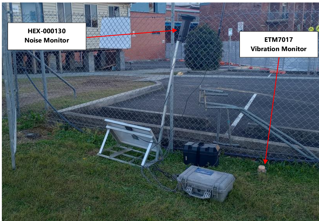
Figure 3 – Noise and Vibration Monitor at North Boundary Near Block A and B
