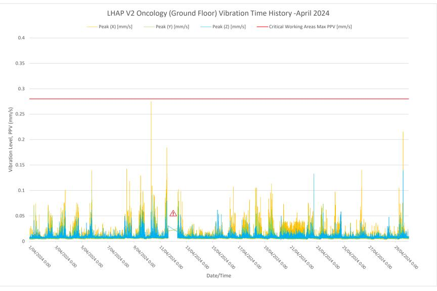
Vibration data unavailable due to planned battery swap over on 11/04/2024. Data between 11/04/2024 at 14:30 hrs and 12/04/2024 at 08:00 hrs and are not included in the April 2024 dataset.
