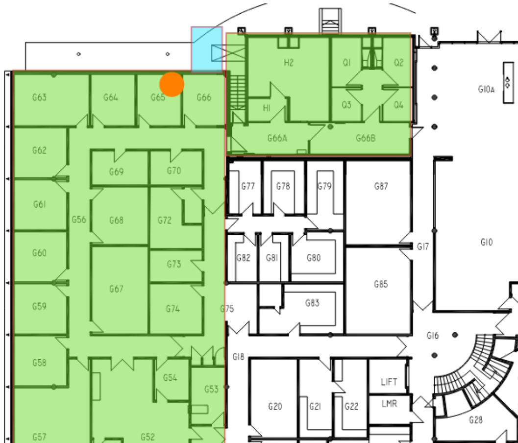
Figure 3: CMRI Animal Holding Facility vibration monitor location
