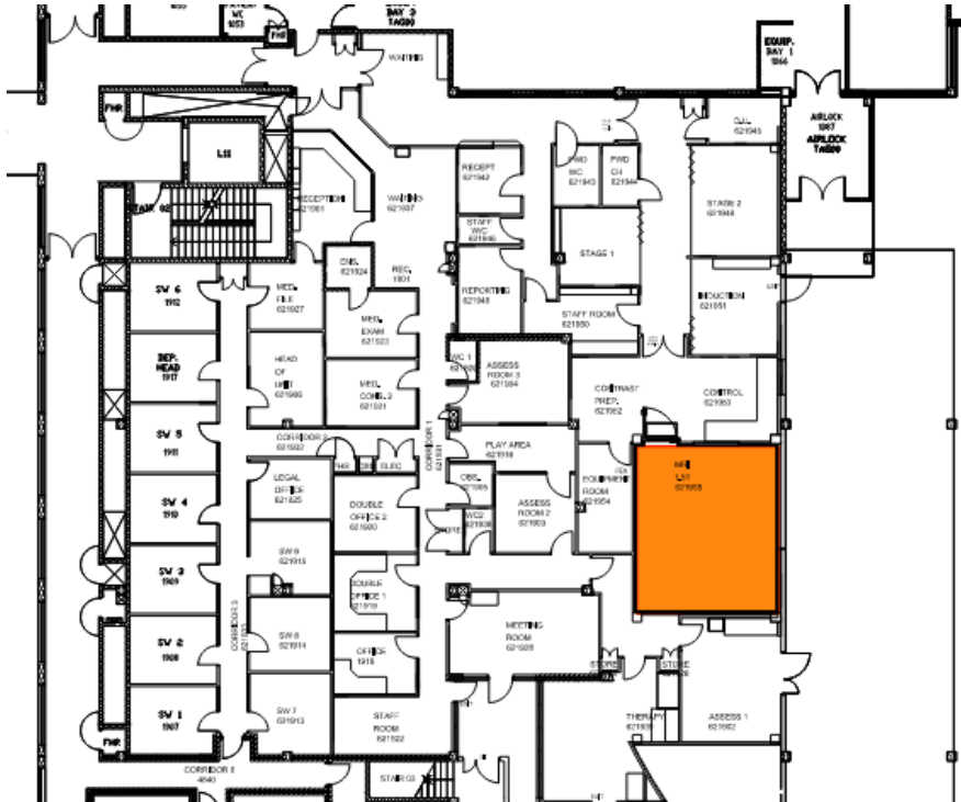
Figure 3: SCHN - 1.5t MRI vibration monitor location
