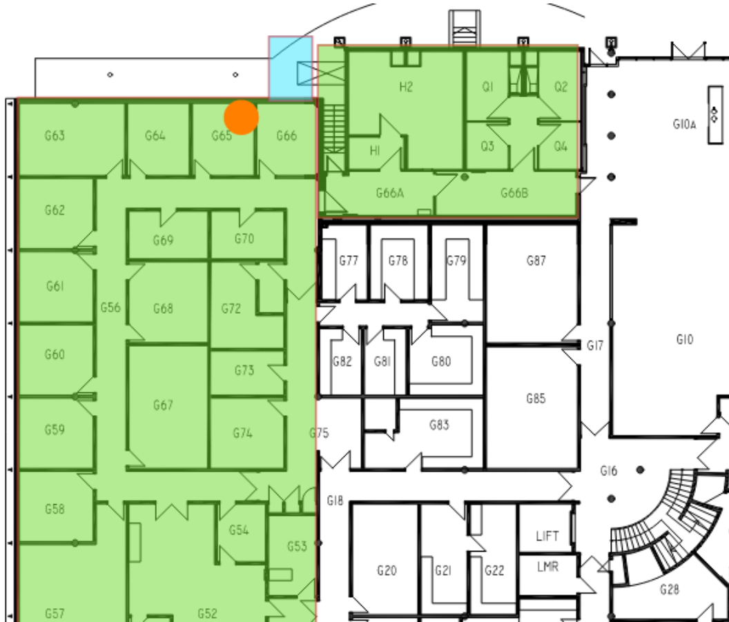
Figure 3: CMRI Animal Holding Facility vibration monitor location
