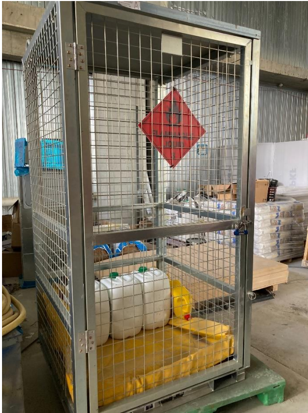
Photo 9 – Locked up cage for storage of flammable chemicals
